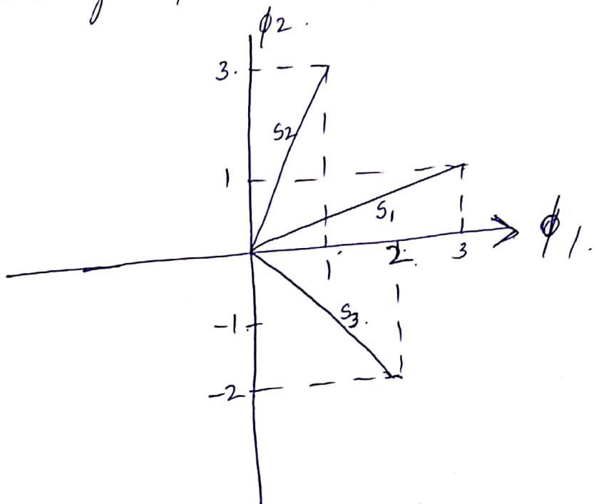
In an-  $N$ - dimensional Euclidean space , we may define lengths of vectors and angles b/w vectors. The length (also called the absolute value or norm) of a signal vector  $s_i$  by the symbol  $\|s_i\|$ . The squared length of an any signal vector  $s_i$  is defined to be the inner product or dot product of  $s_i$  with itself as shown by.
