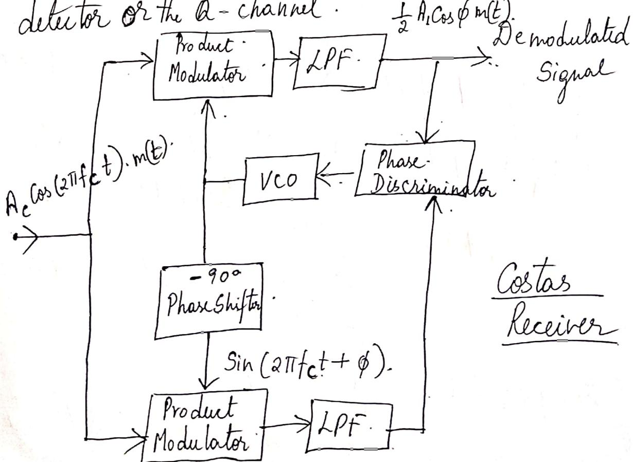
The local oscillator signal is of the same phase as the carrier wave ie  $A_c \cos(2\pi f_c t)$  used to generate the modulated wave. Under these conditions, ~~the~~ I-channel o/p contains the desired demodulated signal  $m(t)$  whereas the Q-channel o/p is zero due to quadrature null-effect of the Q-channel.
